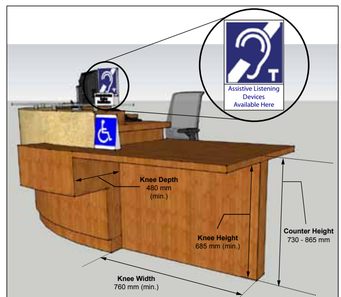
Figure 100: Dimensions of Accessible Service Counter
