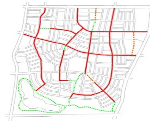
*Figure 10a:* Sidewalks (solid), trails or pathways through parks (dotted), and mid-block walkways (dashed) form a continuous network for pedestrians.
