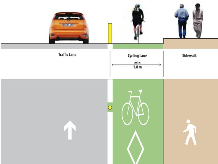
Figure 3-6: Unidirectional laterally separated facility without parking
