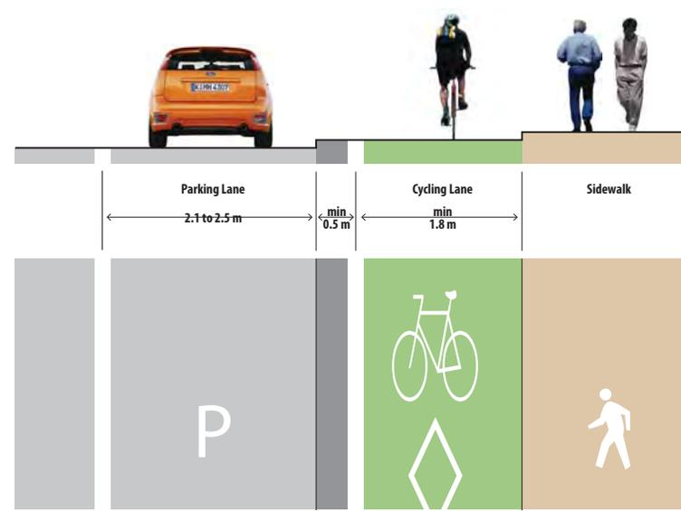
Figure 3-7: Unidirectional vertically separated facility with parking
