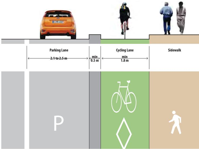
Figure 3-5: Unidirectional laterally separated facility with parking
