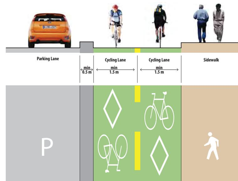
Figure 3-10: Bidirectional laterally separated facility with parking
