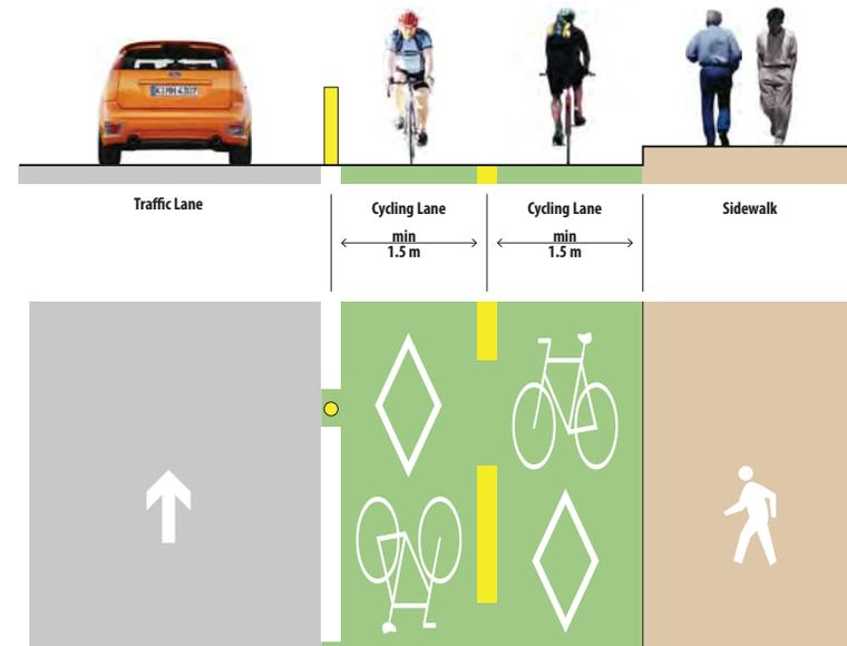
Figure 3-9: Bidirectional laterally separated facility without parking
