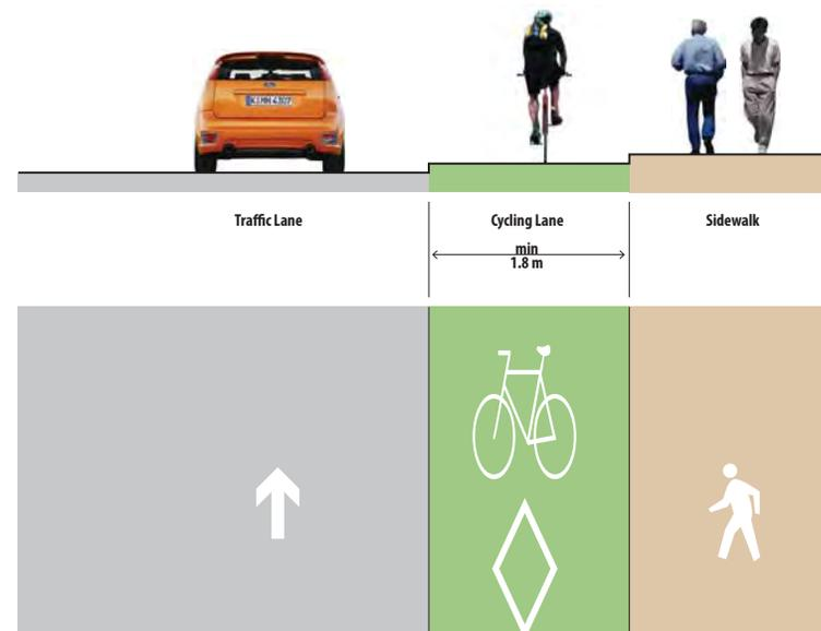
Figure 3-8: Unidirectional vertically separated facility without parking
