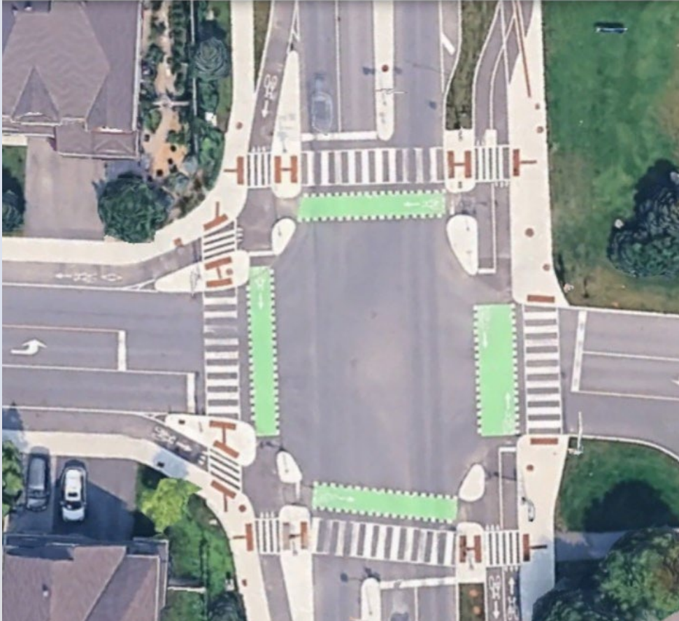
Protected intersection: Highbury Park Drive at Longfields Drive
