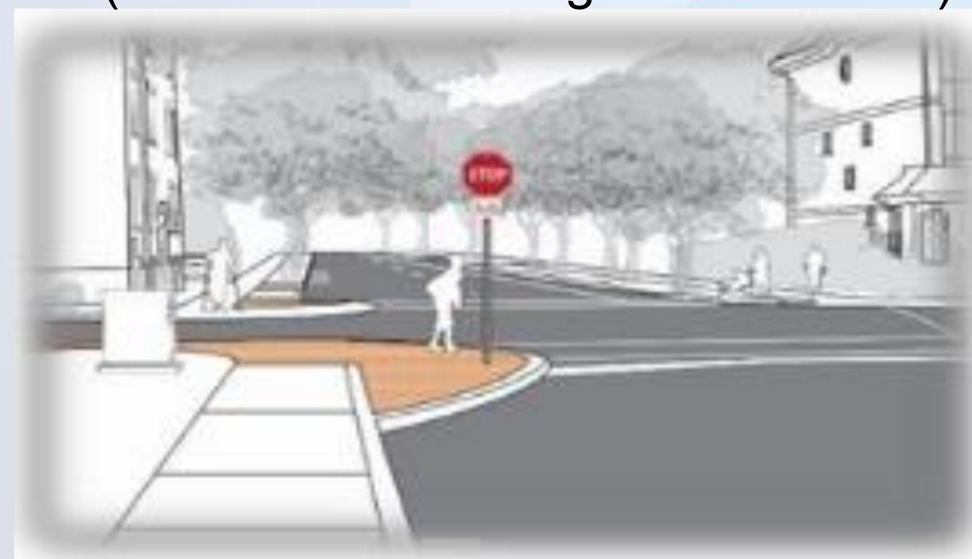
Intersection narrowing (on Ferndale at Churchill) Rétrécissement de l'intersection (sur Ferndale à l'angle de Churchill)
