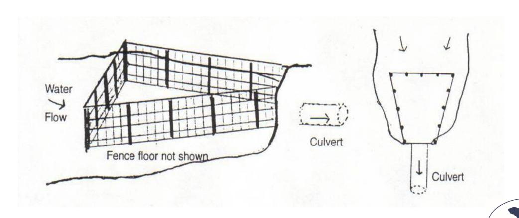
Make the culvert undesirable to dam
