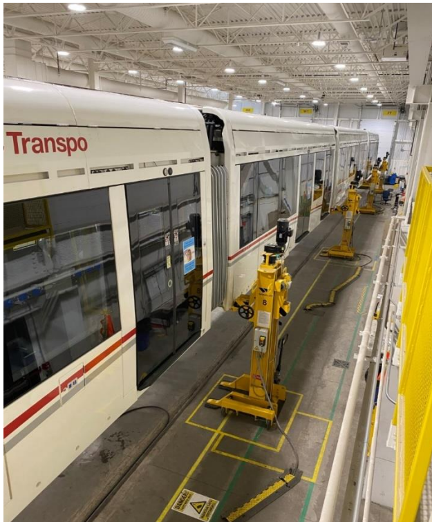
Figure 3.53: Vehicle Lifted by Portable Jacks at MSF2
