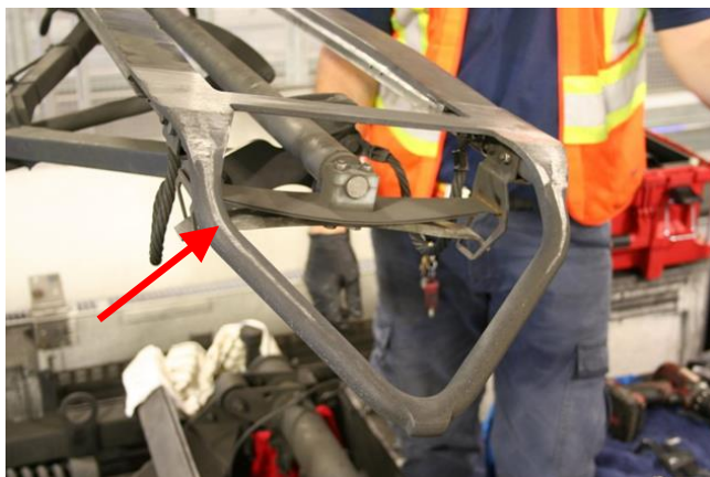
Figure 3.35: Wear on Pantograph Horn
