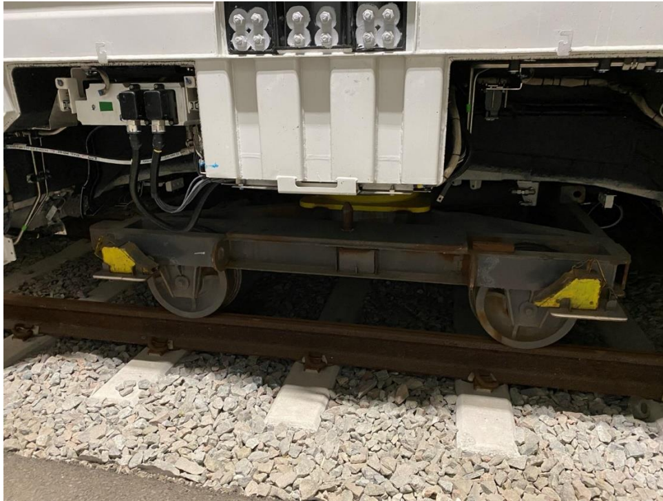
Figure 4.15: Vehicle Missing Trucks
