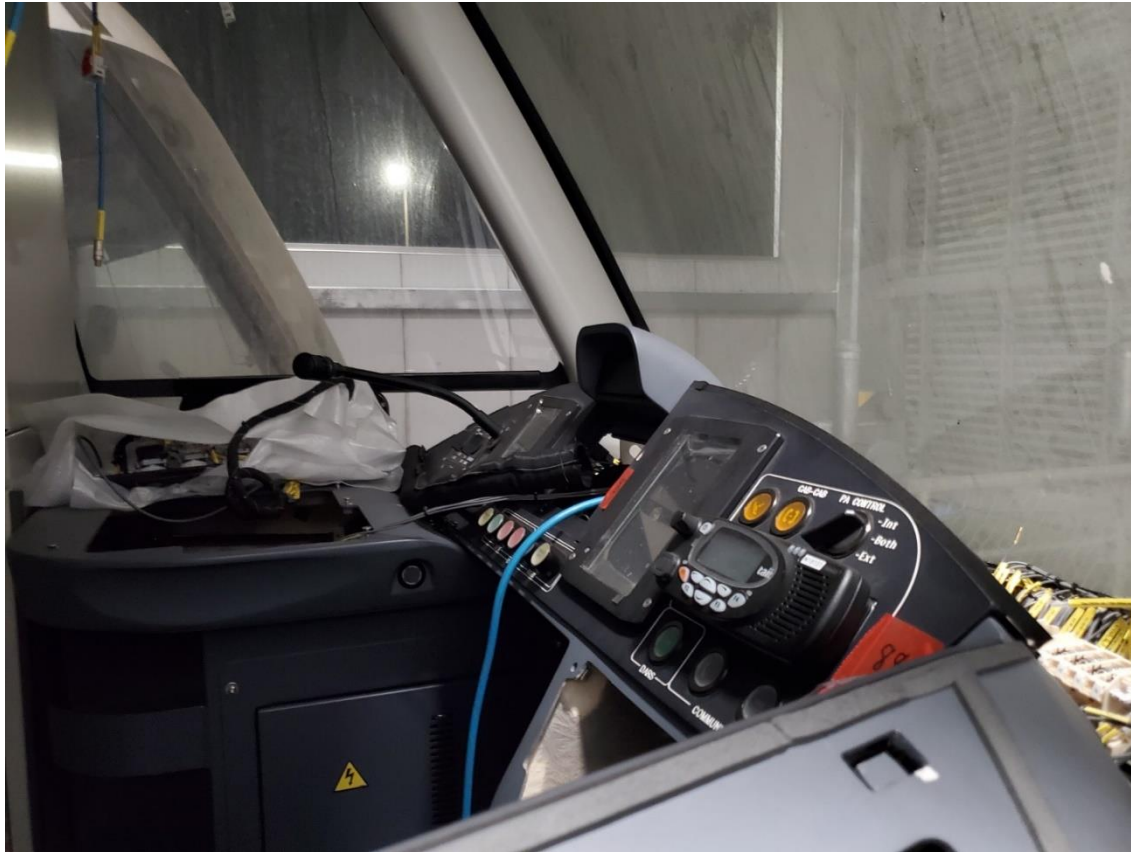
Figure 4.14: Vehicle Missing Cab Components
