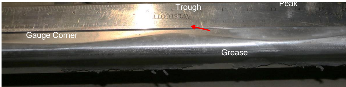
Figure 3.10: Corrugation on High Rail of Curve 220 at 105+115
