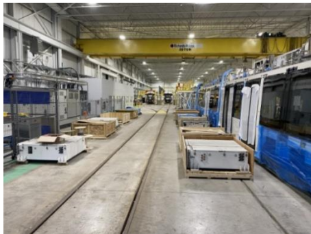
Figure 3.87: APS Units on The Brampton Facility Shop Floor
