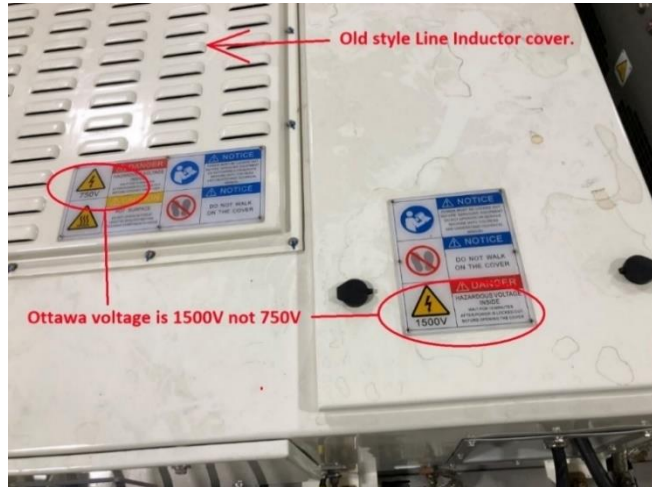
Figure 3.84: Propulsion Converter Indicating the Wrong Voltage and Using the Old-Style Line Inductor Cover
