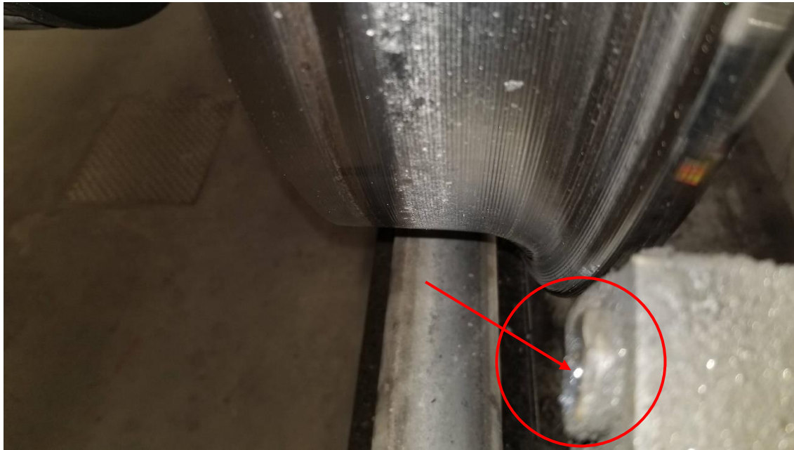
Figure 3.65: Missing Flange Lubrication Spray Nozzle
