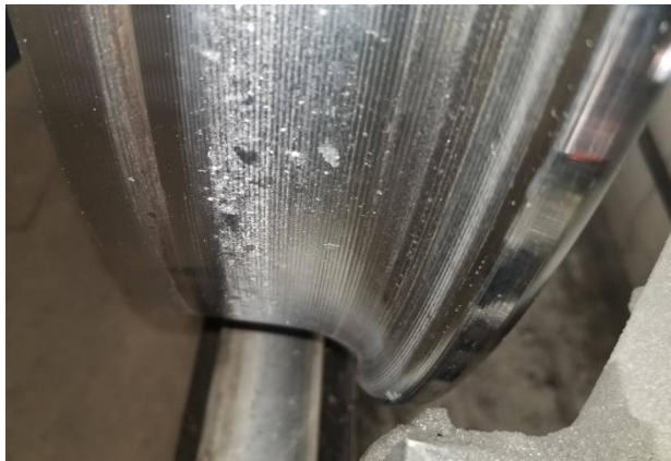
Figure 3.61: Coarse Machining Lines Observed During Site Inspection
