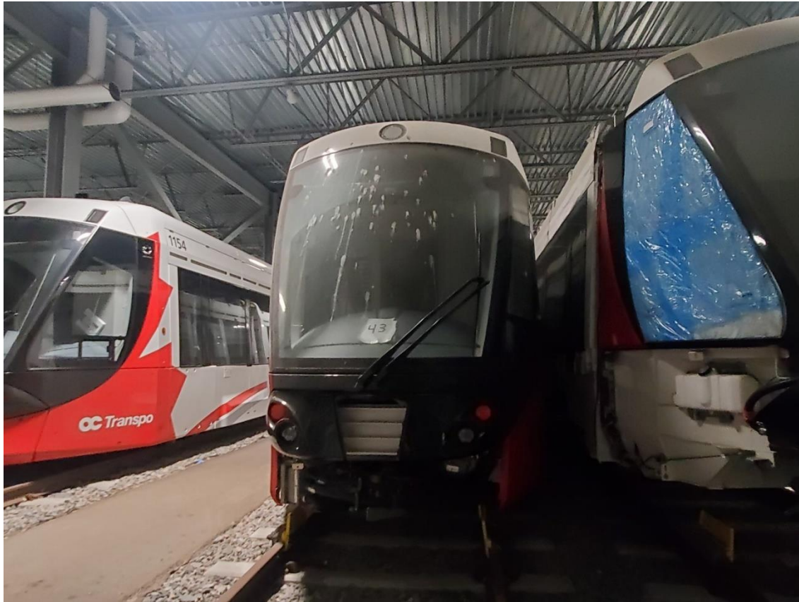
Figure 4.11: Limited Space Available Between Vehicles at the Storage Shed
