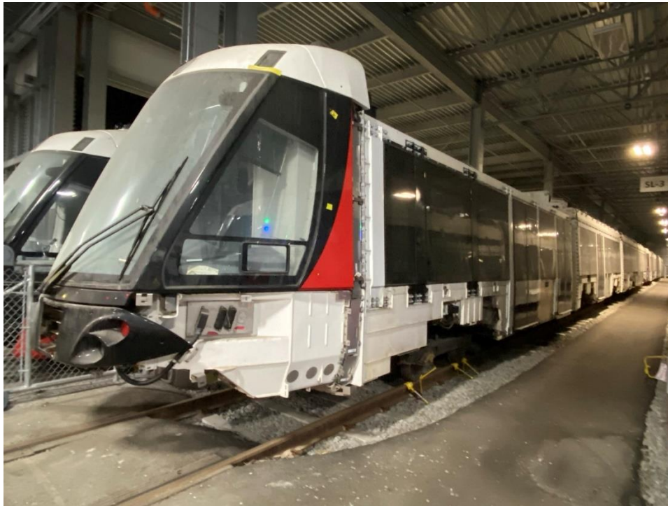
Figure 4.13: Vehicle Missing Side Panels, Coupler, Skirts and Roof Shrouds
