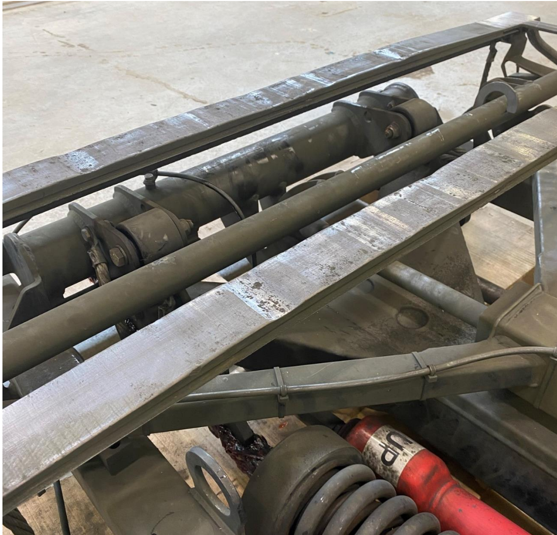
Figure 4.24: Grooved Wear on Pantograph
