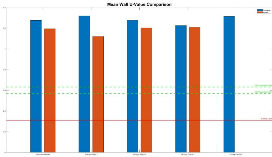
Figure 3: Comparison of Mean Wall U-values of All Buildings against Existing Building Code and EEP
