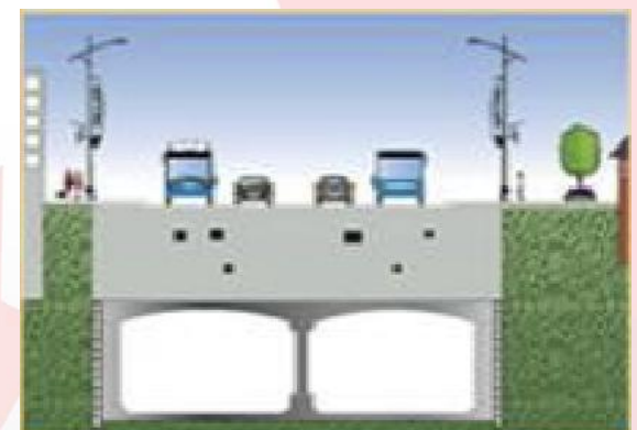
5. Removal of decking/ street restoration
