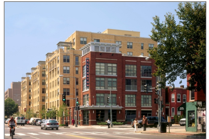
Figure 50: A four- to six-storey streetwall steps back to eight storeys along a main street
