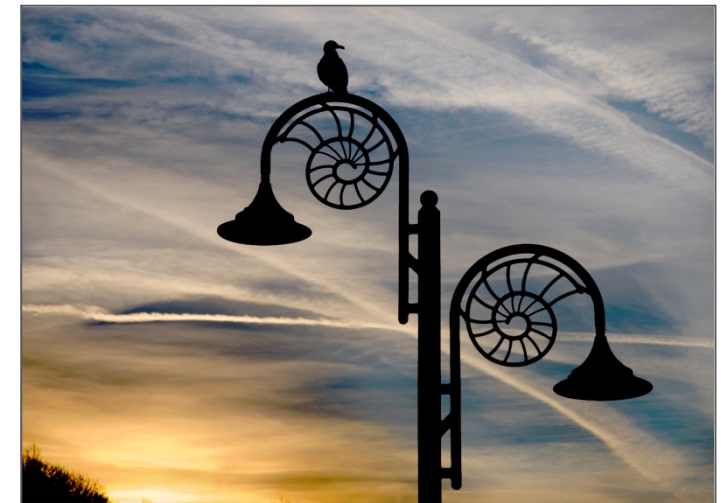
Figure 64: Street and lowered pedestrian-level lighting on a decorative shared post
