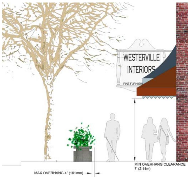
Objects located between 0.7m and 2.0m from the ground should not protrude more than 100mm
