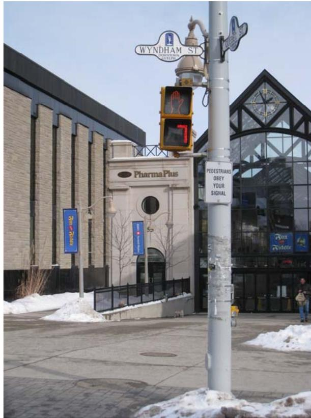
Pedestrian countdown signal head with the flashing “DON’T WALK” hand above the seconds remaining until the solid “DON’T WALK” Location: Guelph, ON. Source MMM Group
