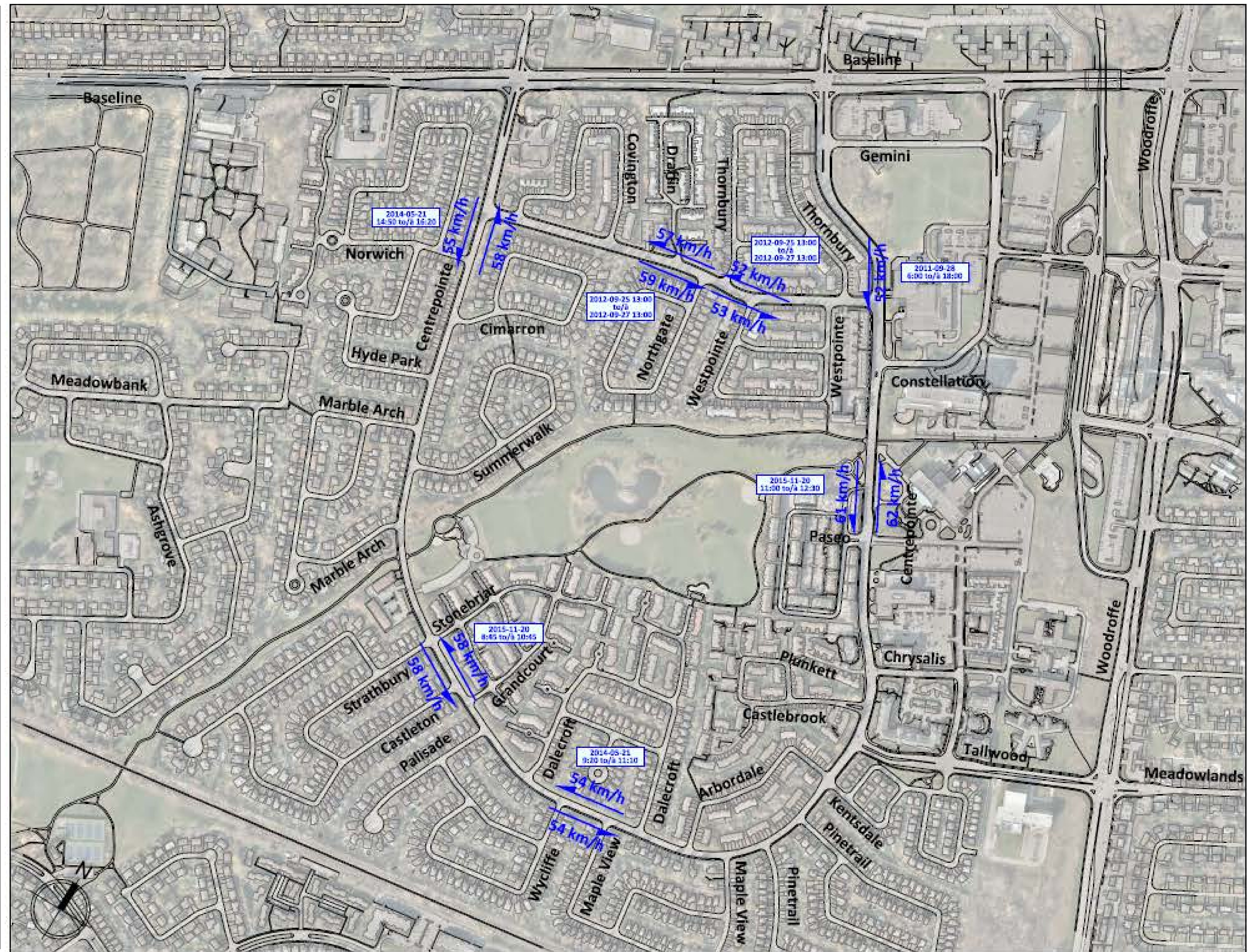
CENTREPOINTE DRIVE AND HEMMINGWOOD WAY AREA TRAFFIC MANAGEMENT STUDY 85th Percentile Speed (km/h)
