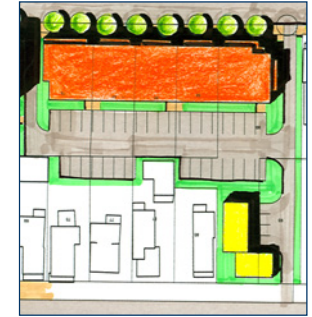
An example of commercial parking at the rear of a residential lot that abuts a mainstreet property
