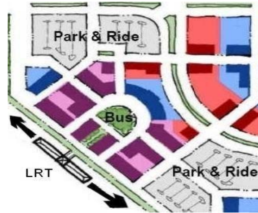
Figure 45a: Transit-oriented development opportunities increase at park & ride stations when vehicle parking is located in close proximity, but not immediately adjacent to the station.
