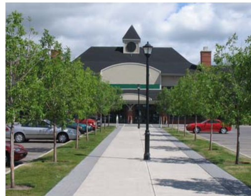
Figure 38: Separate vehicle and pedestrian functions within parking lots for safety and aesthetic reasons.
