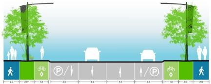
PROPOSED CONDITION - ELEVATED SECTION AMÉNAGEMENT PROPOSÉ - COUPE EN ÉLÉVATION
