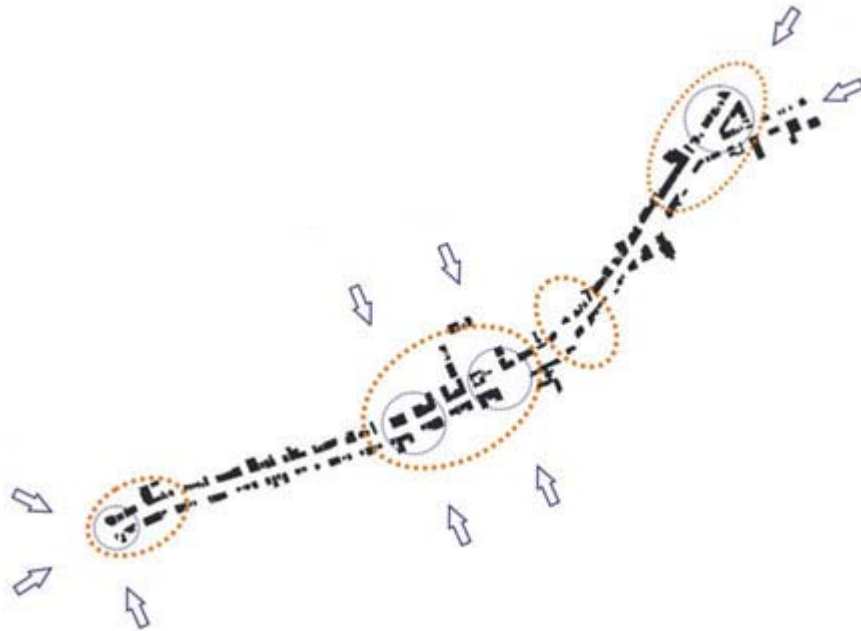
Figure 3-5: Gateways and nodes at key routes entering the mainstreet corridor.
