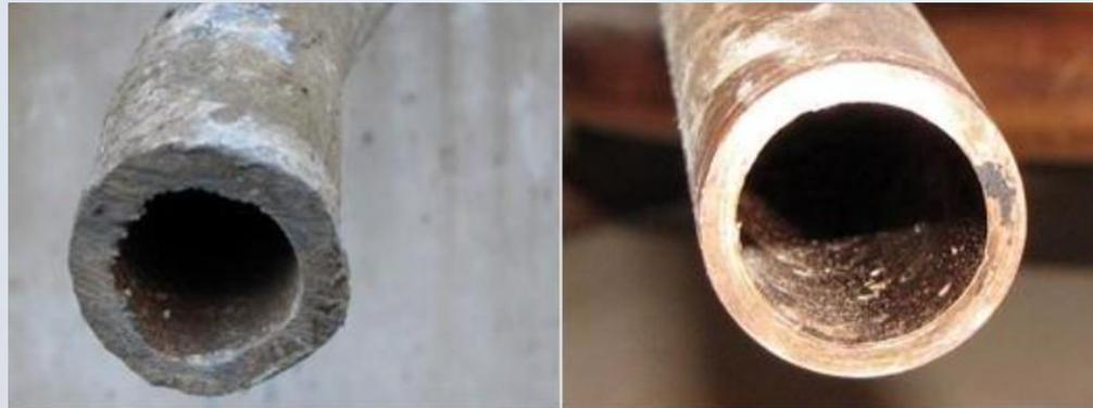
Lead pipe (left) & copper pipe (right)
