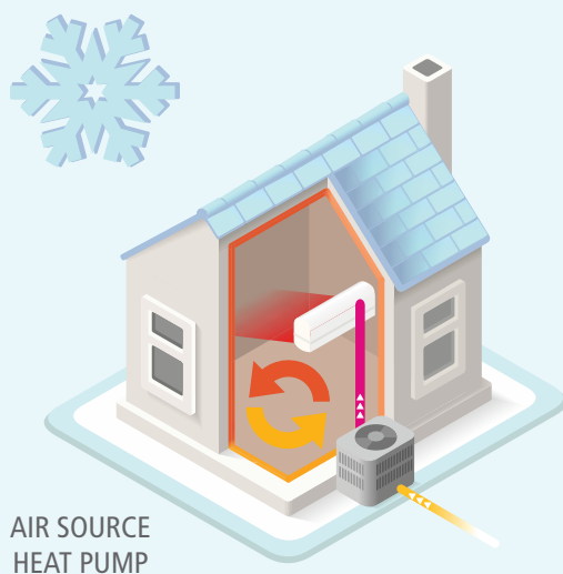
Figure 6: Comparison Schematics of Ground and Air Source Heat Pumps.
