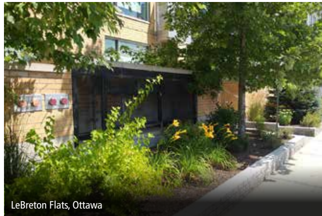
Figure 3-16 Integrate gas metres and other utilities into architecture and landscaping design.
