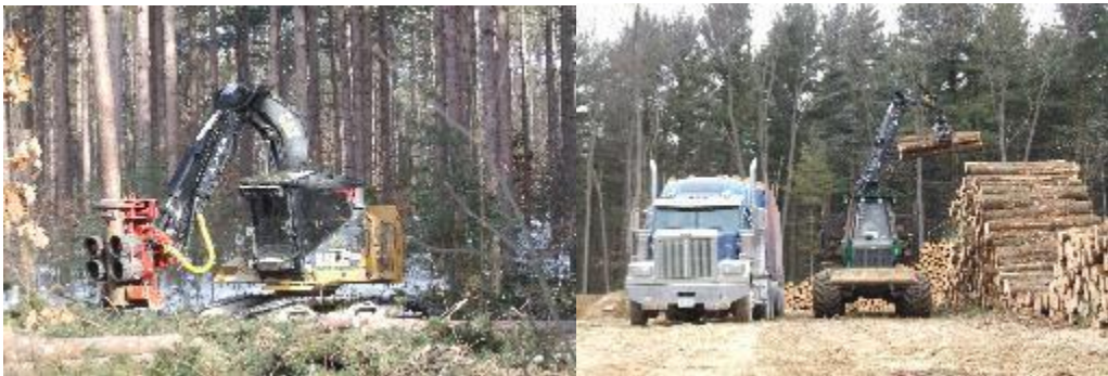
Figure 28. (Left) A single-grip harvester fells and processes a mature red pine. (Right) A forwarder brings the products to the landing and loads them onto a haul truck.
