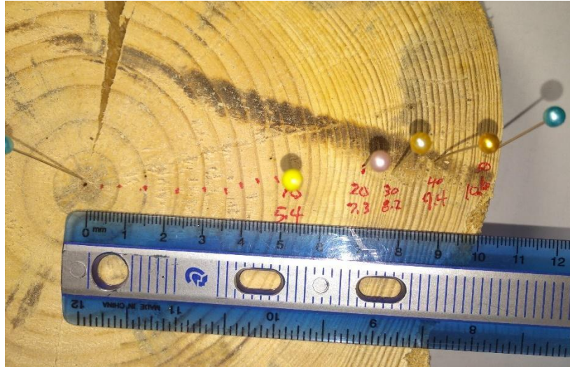
Figure 9. Photo of 1.0m cookie with pins inserted at 10-year increments from the centre of the tree. Note the rapid decline of diameter growth after Age 20
