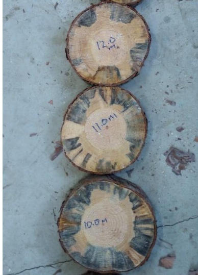
Figure 15. Photo from stem analysis tree showing blue stain decay
