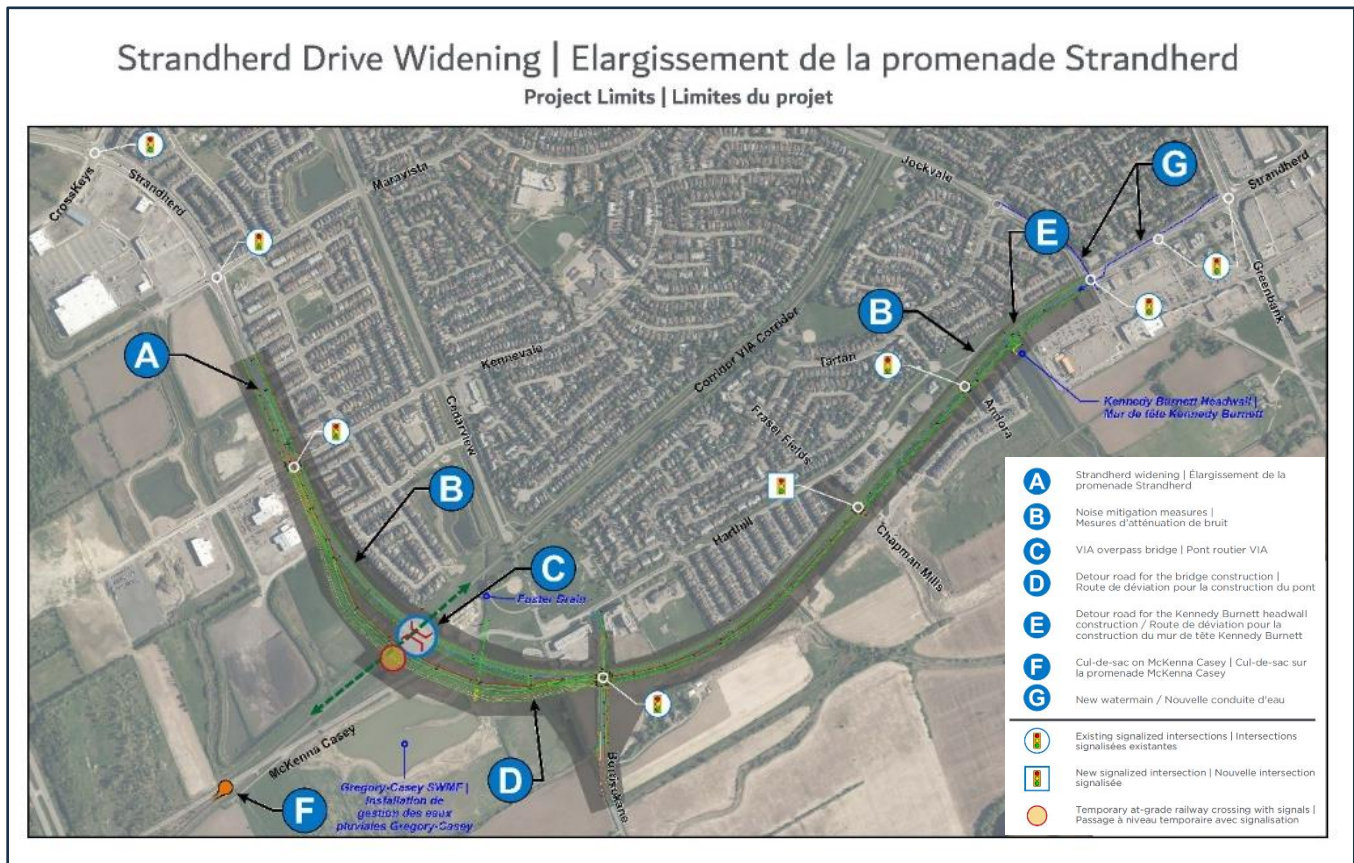
Figure 7: Strandherd Drive Widening and Realignment (Project Overview)
