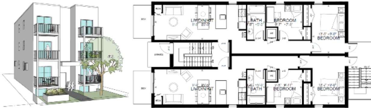
Figure 8: Building illustration and floor plans for one configuration of eight, two-bedroom units on a 12m wide lot.
