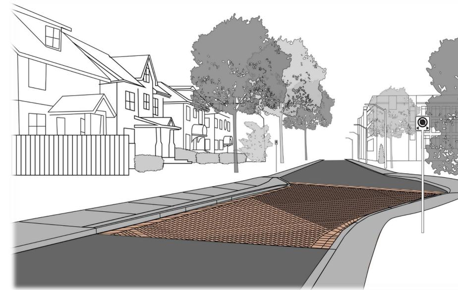
**Textured surfaces** contrast typical asphalt pavements used on City roadways
