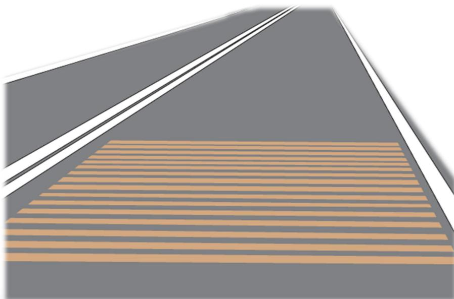
**Transverse rumble strips** are raised buttons, bars, or recessed grooves closely spaced on the roadway that create both noise and vibration in a moving vehicle
