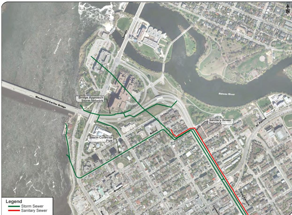
Figure 10: Major Storm and Sanitary Sewer Alignments – North End
