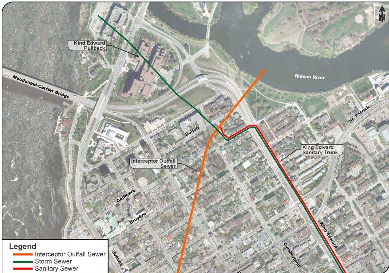
**Figure 24: Interceptor Outfall Sewer, King Edward Sanitary Trunk and Pull Back**
