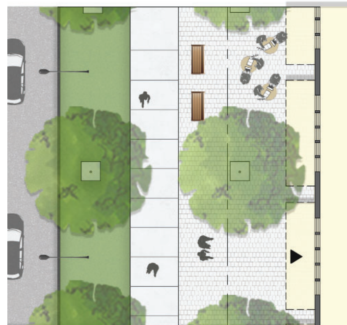
Diagram 8: Streetscape section and plan showing the boulevard, sidewalk and area for retail amenity (frontage zone).
