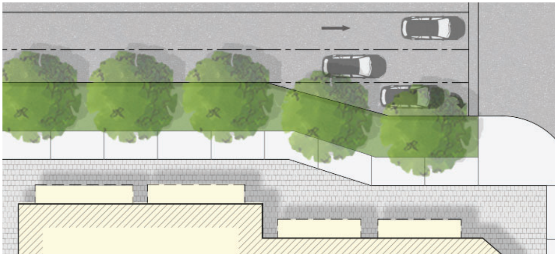
Diagram 9: Turn lanes do not diminish the consistency of the sidewalk and landscape areas.
