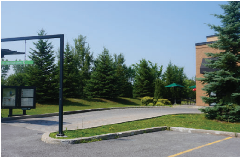
Figure 11: A grassed curb separates the stacking lane from parking areas in this drive-through site.
