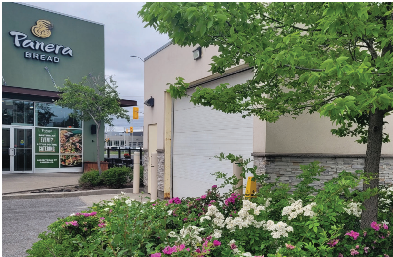
Figure 13: At this drive-through development, the garbage enclosure structure is visually harmonized with the main building through similar material colour and texture.
