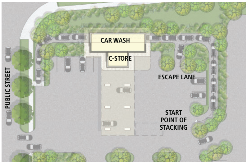
Diagram 3: The escape lane allows cars to get out of a queue.
