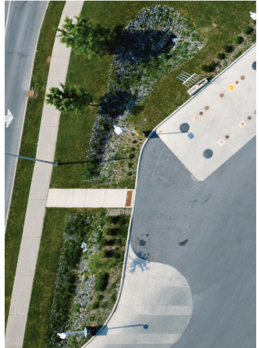
Figure 22: The planting bed collects and stores stormwater to reduce stormwater runoff.
