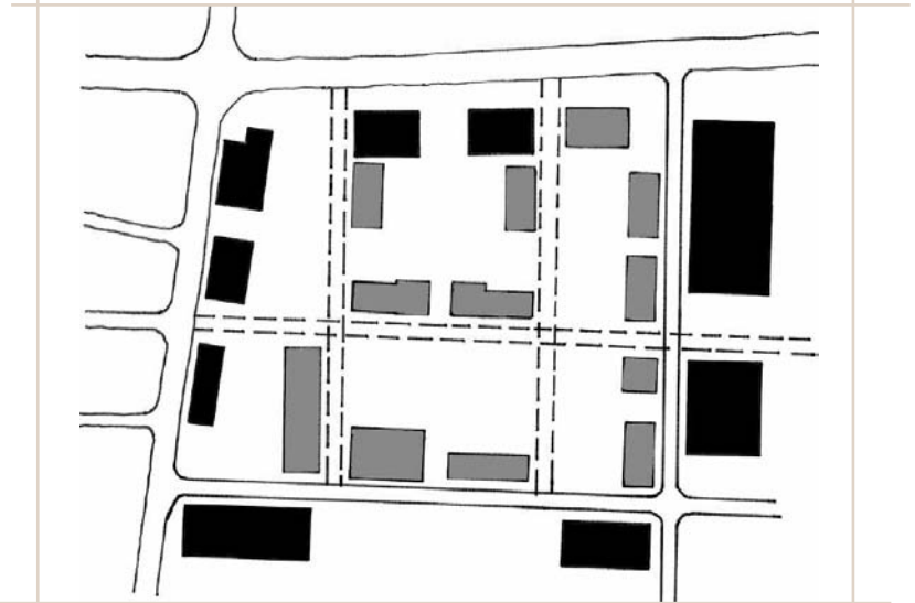
Figure 8: Basing new development on a grid layout can easily accommodate redevelopment and future intensification.
