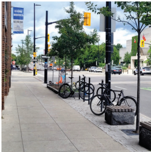
Figure 20: Provide unobstructed pedestrian clear zone and a boulevard for street furniture and trees.
