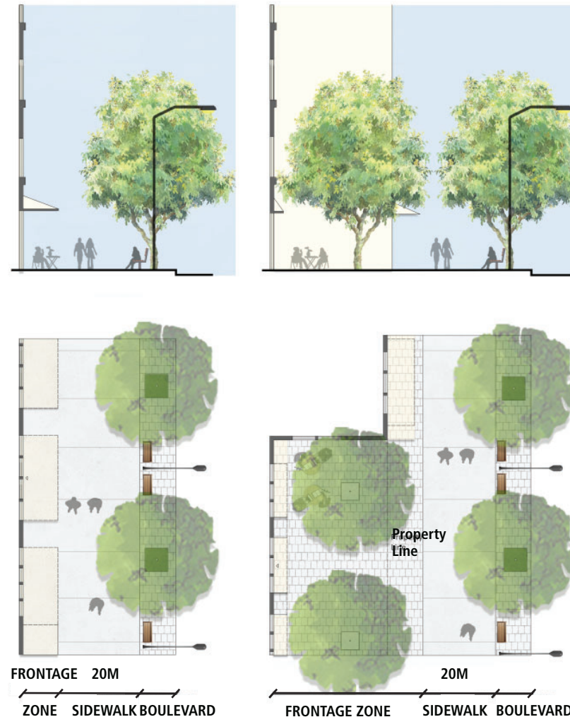
Diagram 4: Streetscape section and plan showing the boulevard, sidewalk and area for retail amenity (frontage zone).
