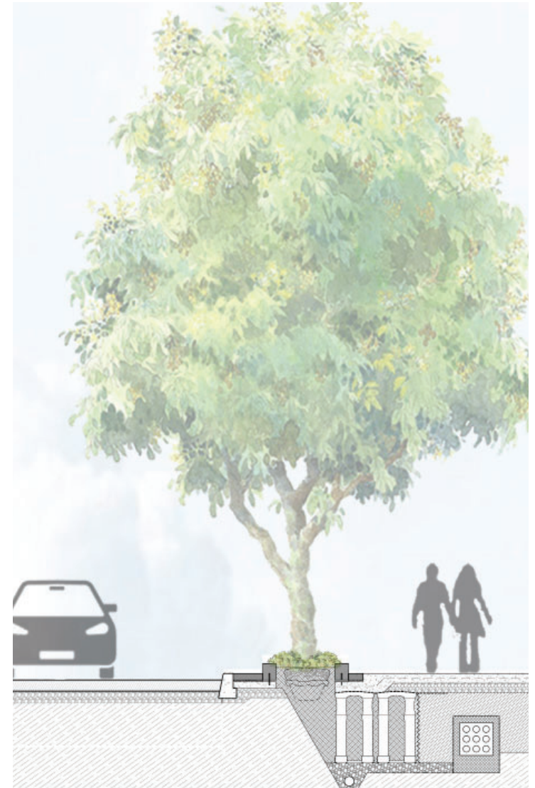
Diagram 5: Silva Cell is one of the methods to plant trees in area of constraints. This design adapts from the general Silva Cell concept.
