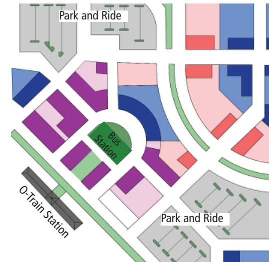
Diagram 2: Transit-oriented development opportunities increase at park & ride stations when vehicle parking is located in close proximity, but not immediately adjacent to the station.
