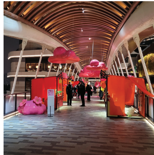
Figure 27: This grade separated pedestrian connection includes retail services that help to generate pedestrian activity and avoids a "tunnel" feeling.
