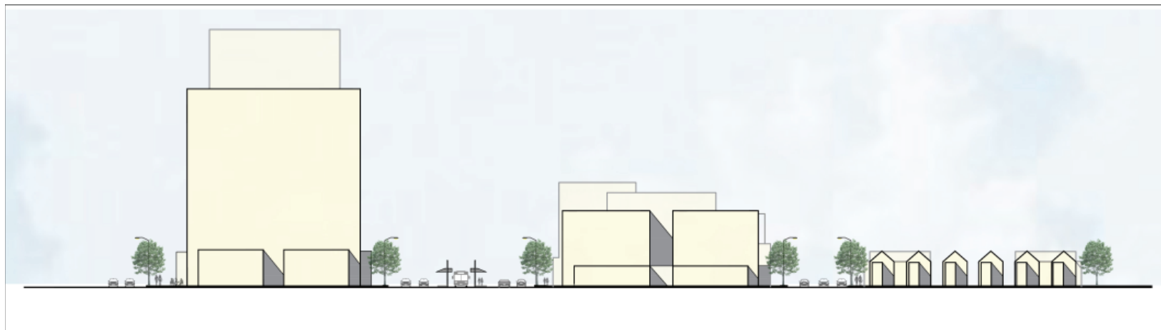
Diagram 11: A transition in building scale protects the adjacent residential neighbourhood and enhances the ability of the station to become part of the neighbourhood.
