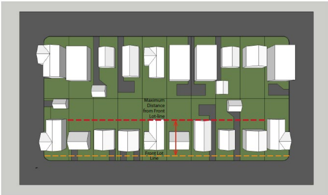
--- Maximum Building Distance from Front Lot Line
