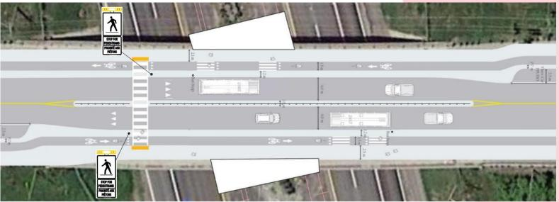
Plan view reflecting the connectivity enhancements along Orleans Blvd, with a new cycle tracks in both directions, and a pedestrian crossing with flashing beacon lights and overhead signs to alert vehicles. The cycle tracks and new sidewalks will be constructed to the north to Fortune Drive & Sugar Creek Way, and to the south to Lumberman Way.
