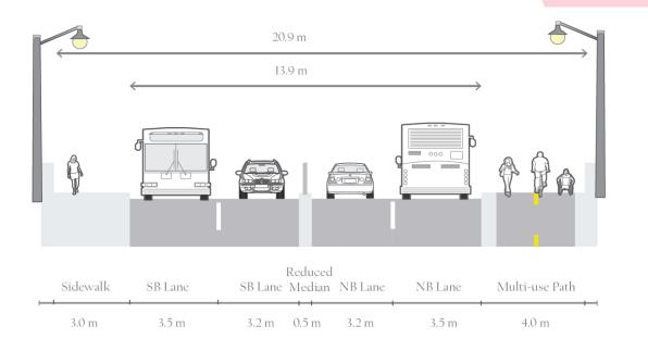
Cross-section looking toward the north, demonstrating the connectivity enhancements described in the previous slide, with the Multi-Use Pathway reflected along the northbound lanes.
