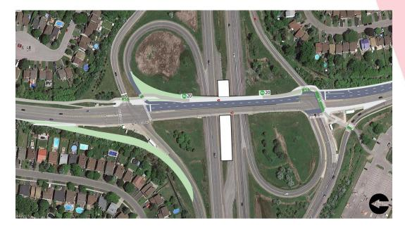
Plan view reflecting the connectivity enhancements along Jeanne d'Arc Blvd, with a new Multi-Use Pathway being constructed along the northbound lanes leading toward the bridge from both the north and south.
