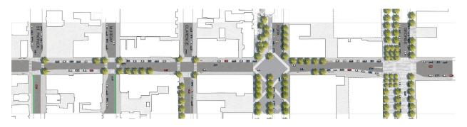
A special paving treatment across the onstreet parking areas, which are raised to near the sidewalk level with low curbs
