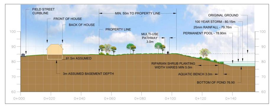
Cross Section B-B: Typical cross section near Field Street
