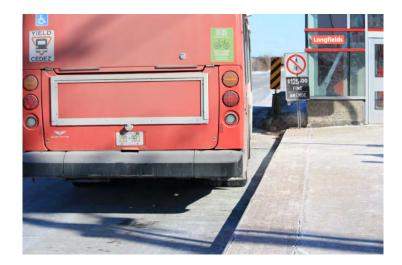
Remove the concrete barriers with a blunt end from the travel lane. Or install a TL-3 F-Shape concrete barrier along the edge of the platform with a pedestrian railing 1000mm high of appropriate length of need and taper to shield passengers on the platform from the swept path of the articulated bus.
