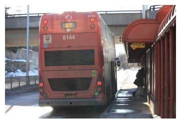
Either reduce operating speed of buses to 20 km/h within the limits of the station to mitigate severity of possible collision with canopy or alternatively remove the canopy.
