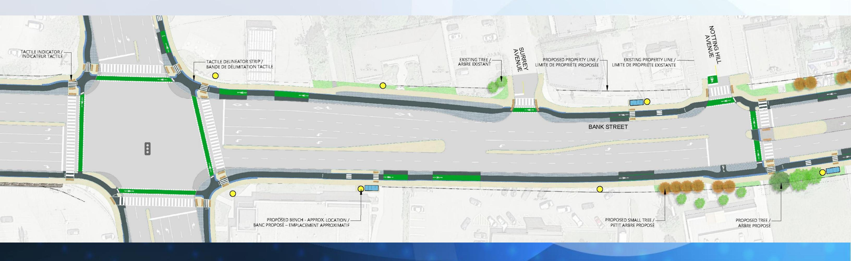
Proposed pedestrian signal on the south leg of the Notting Hill intersection with a bi-directional cross
