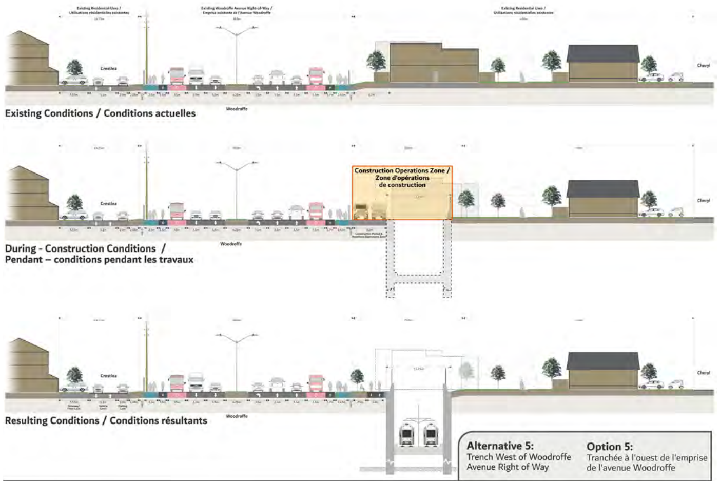
Figure 6-12 Alternative 5: Trench West of Woodroffe Avenue Right-of-Way
