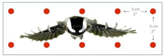
Figure 6: The spacing of markers is representative of the area occupied by a flying songbird, the most numerous victims of collisions (American Bird Conservancy / Safe Wings Ottawa).
