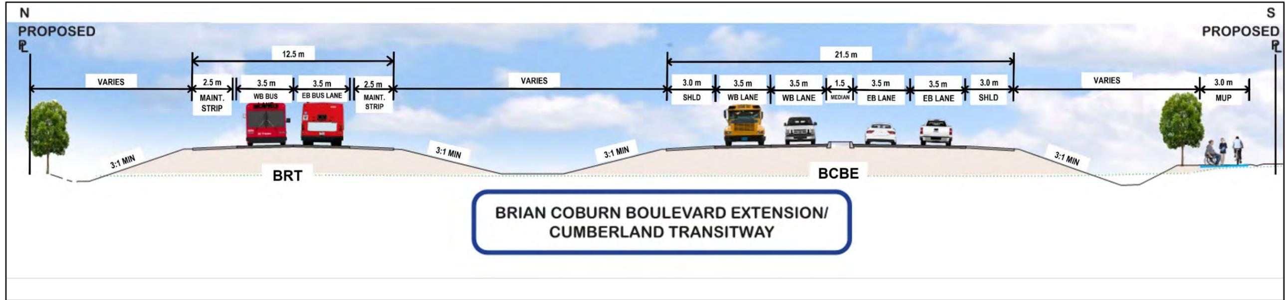
Figure Ex-7: Recommended Plan – Typical Cross-Section
