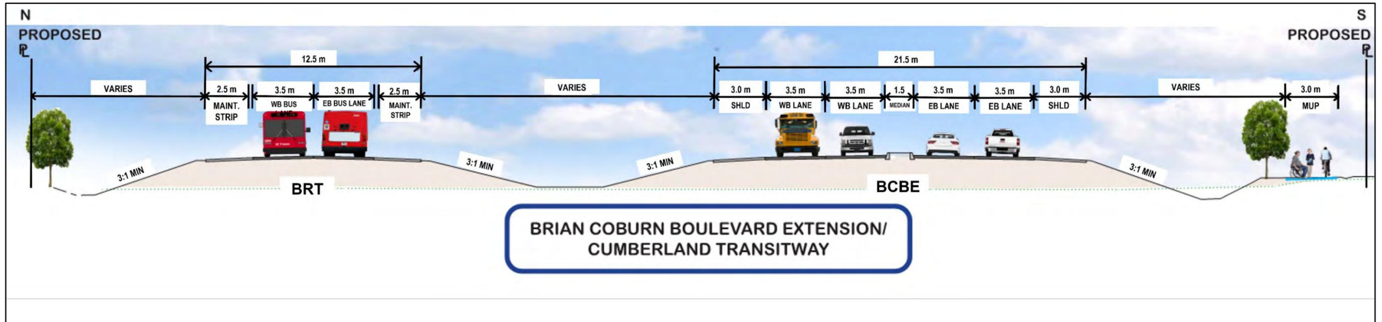
Figure 8-2: Recommended Plan - Typical Cross-Section
