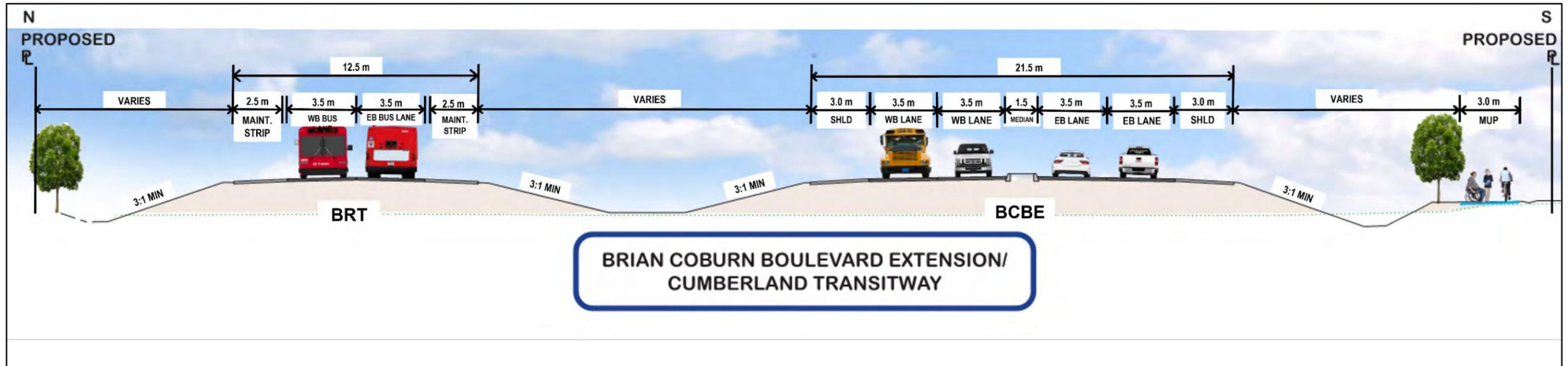
Figure 8-2: Recommended Plan - Typical Cross-Section
