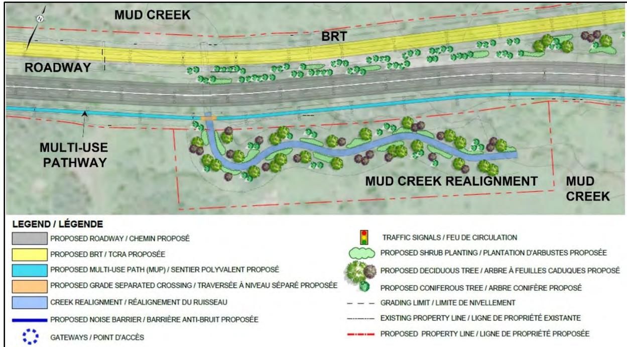
**Figure Ex-10: Mud Creek Realignment**
