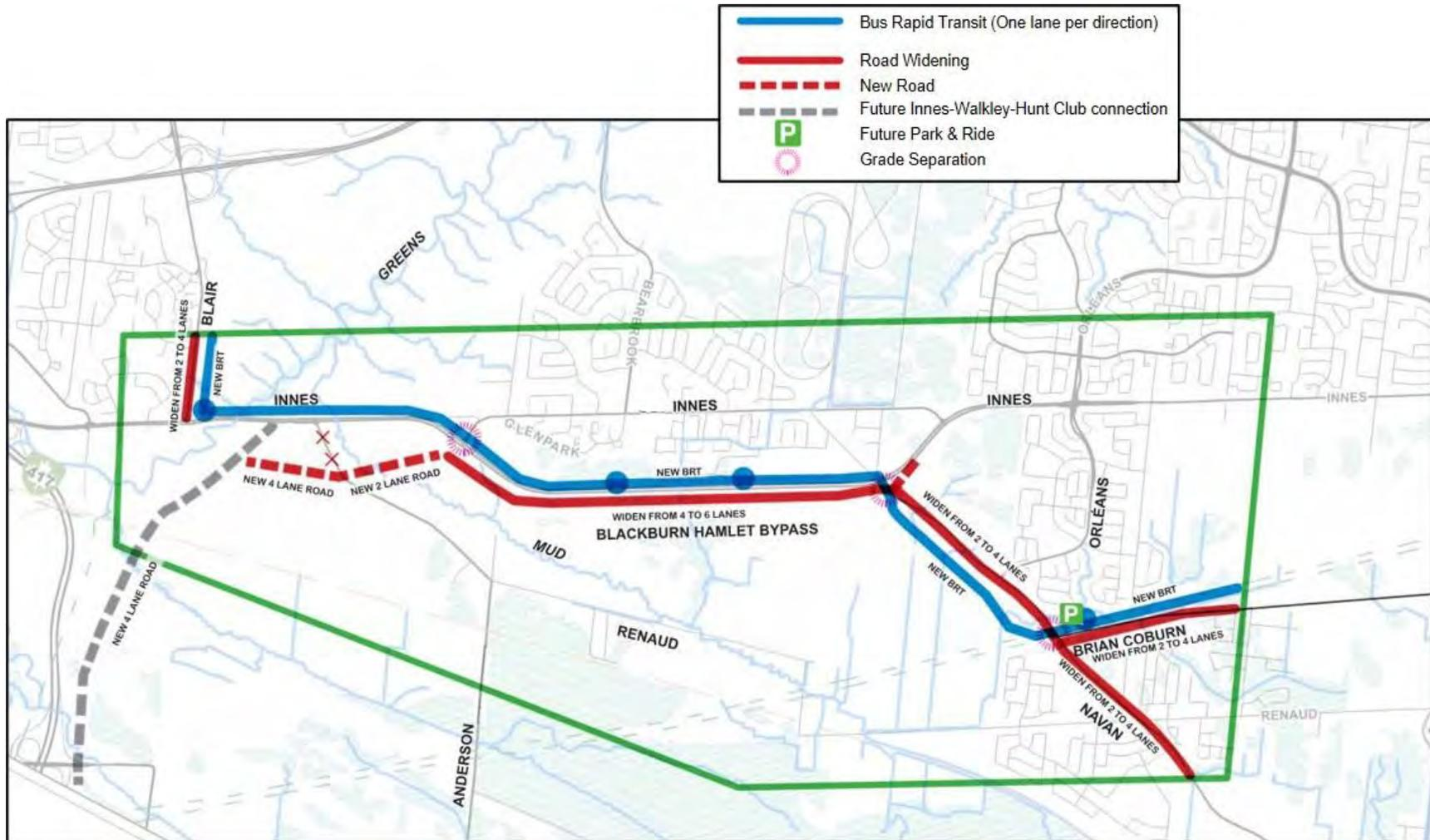
Figure 6-7: Option 4 - Widen Navan/BRT off Navan
