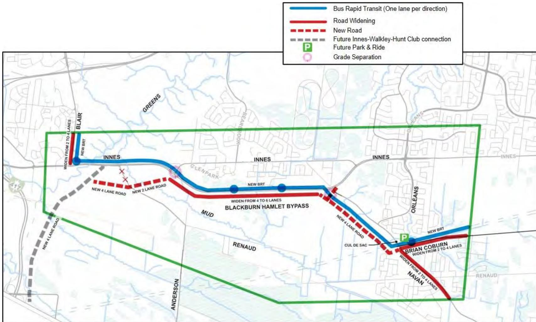
Figure 6-4: Option 1 - New Road & BRT off Navan
