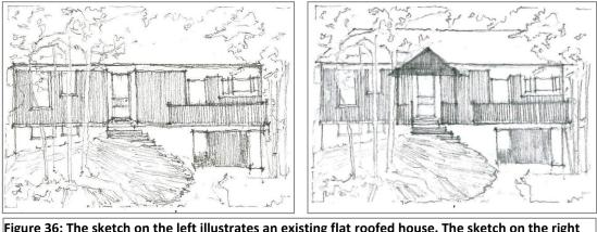
Figure 36: The sketch on the left illustrates an existing flat roofed house. The sketch on the right illustrates an inappropriate alteration to the original building (addition of a gable roof). Sketch by: Blessy Zachariah
