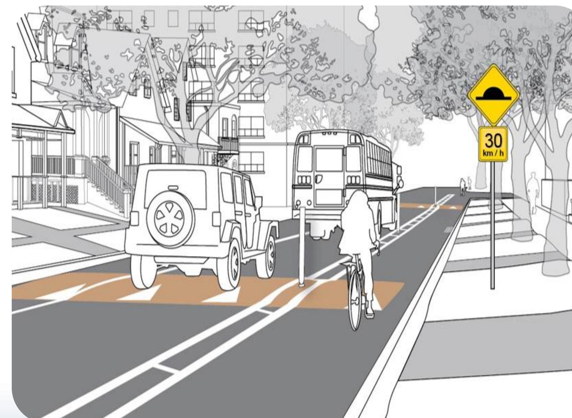
**Speed humps** are raised areas of the roadway, which cause vertical upward movement of traversing vehicles.
