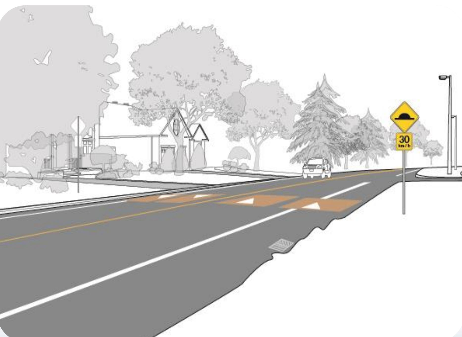
**Speed cushions** are raised areas, similar to speed humps, but not covering the entire width of the road. They are designed to allow large vehicles to "straddle" the cushions, while smaller vehicle are vertically deflected.
