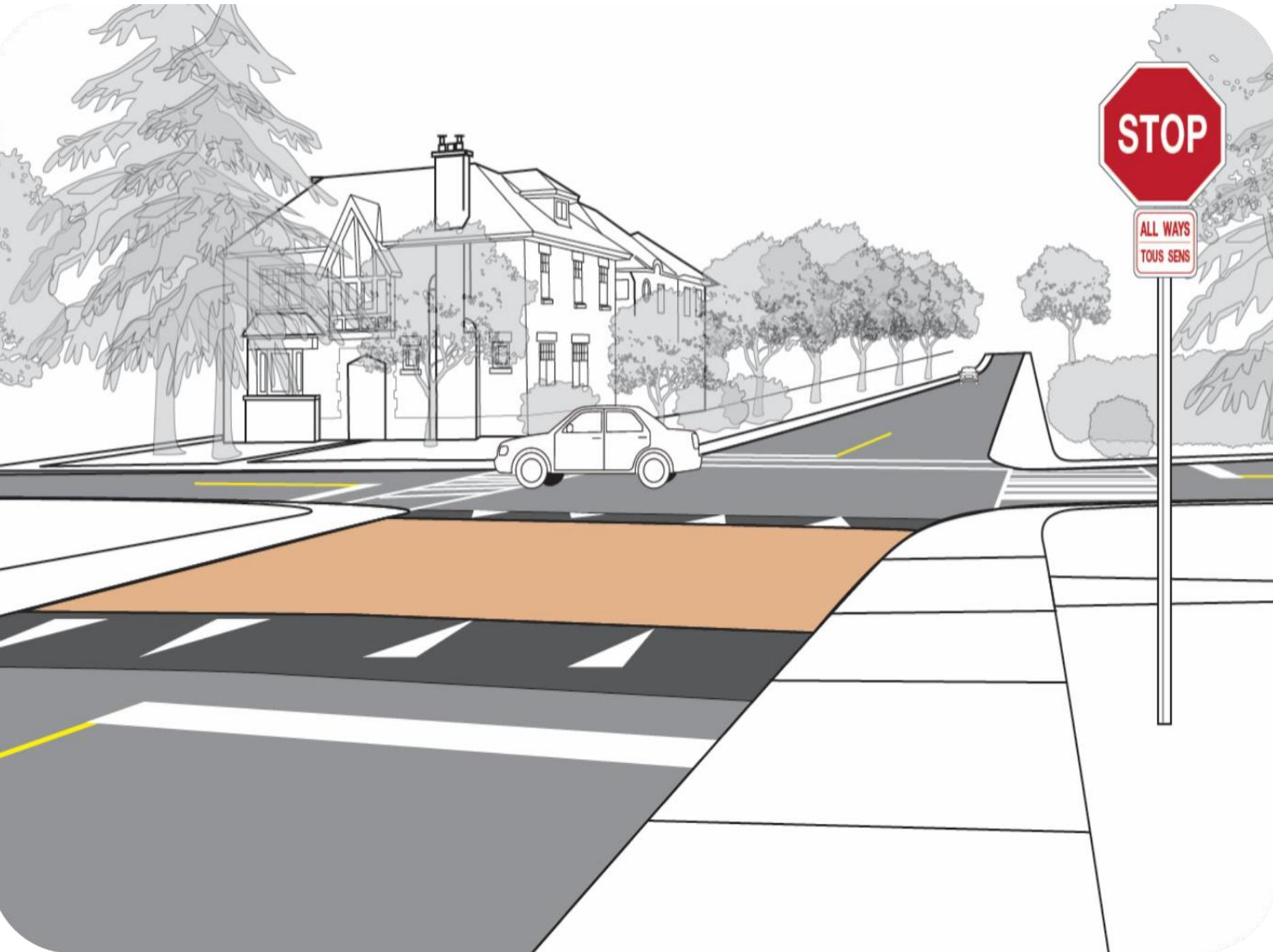
**Raised crossings** are marked pedestrian and / or cycling crossings at intersections, or mid-block locations, constructed at a higher elevation than the adjacent roadway.
