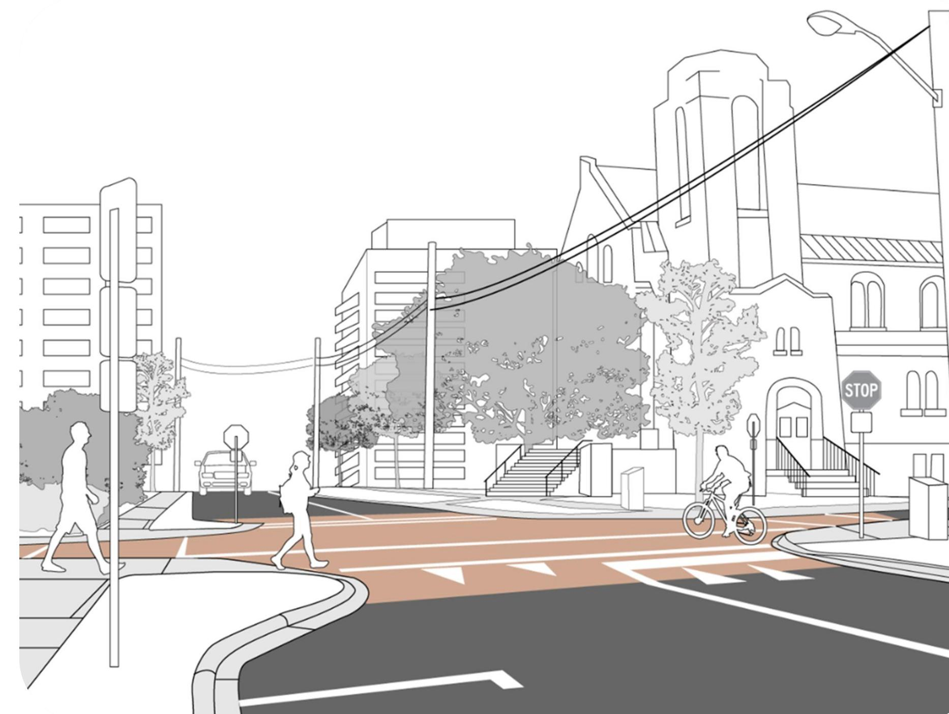
**Raised intersections** are intersections constructed at higher elevations than the adjacent approach roads.
