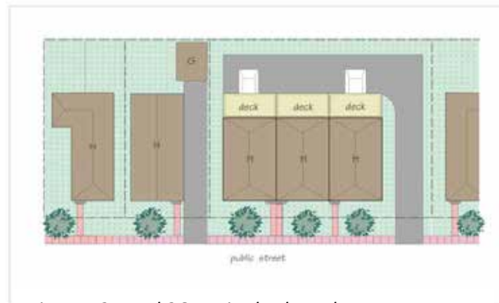
Figures 25 and 26: A single shared access driveway for multiple units matches the neighbourhood pattern of parking at the back. A single vehicular access reduces vehicle/pedestrian conflict, allows for more soft landscaping in the front yard, and permits more on-street parking.
