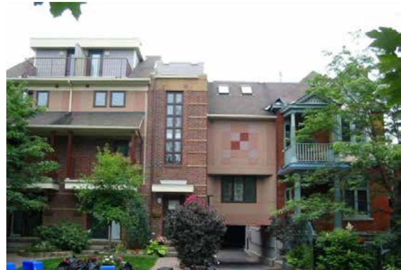
Figure 27: The design of this infill minimizes the impact of car storage by locating shared parking behind the development, internal to the site and accessed through a low entryway.
