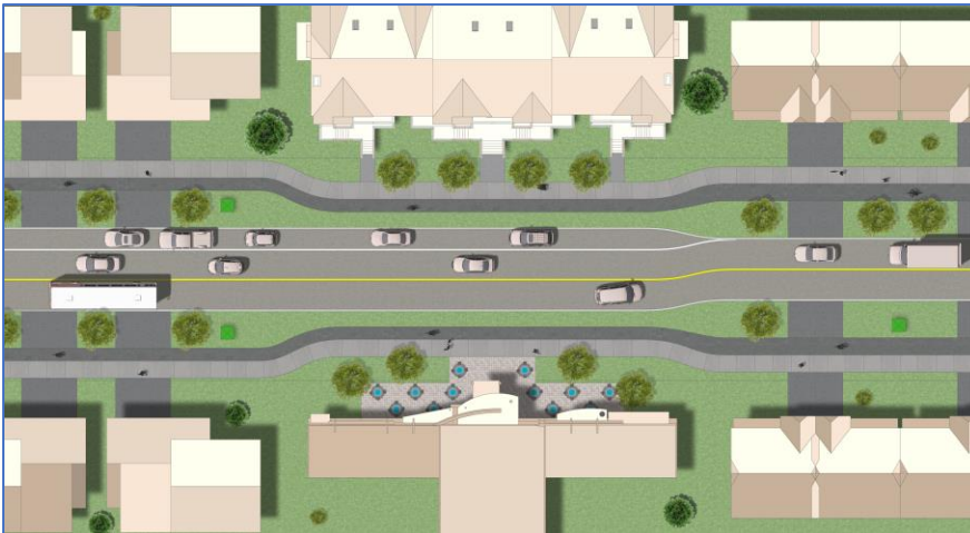
Figure 16 Various cross-section designs can be used along a corridor to respond to the land use context and the transportation functions (not to scale)
