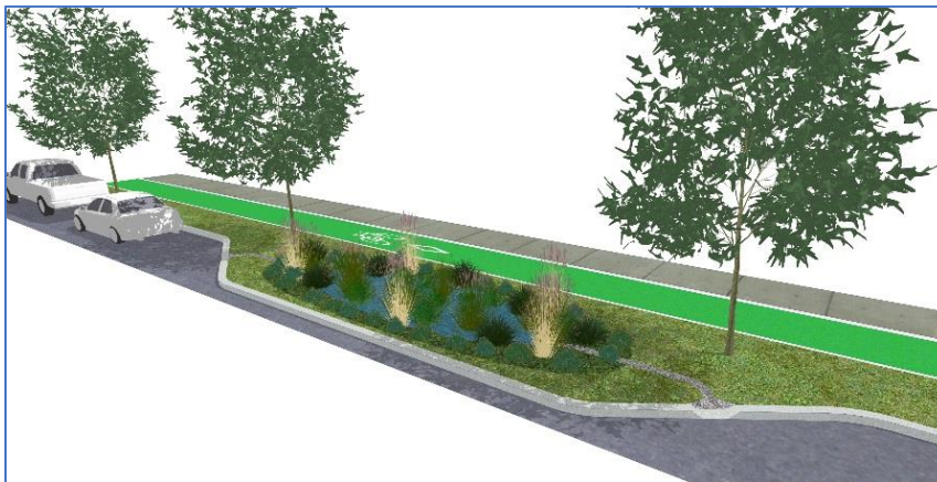
Figure 24 Bulb-outs can provide added space for bio-swales
