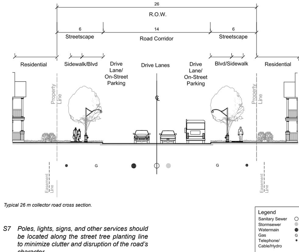
Typical 26 m collector road cross section.
