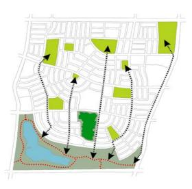
Figure 7a: Stormwater management ponds can be important contributors to the overall greenspace network.
