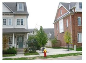
Figure 46b: A 6.0 metre walkway corridor provides a comfortable walking space and privacy for adjacent properties, while still maintianing sightlines for visual surveillance.
