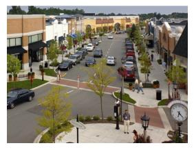
Figure 28b: Sidewalk "bulb-outs" and tighter corner radii reduce vehicle turning speeds and minimize crossing distances for pedestrians.
