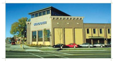
Figure 12: Wall projections and colour/material changes reduce the perception of building size.
