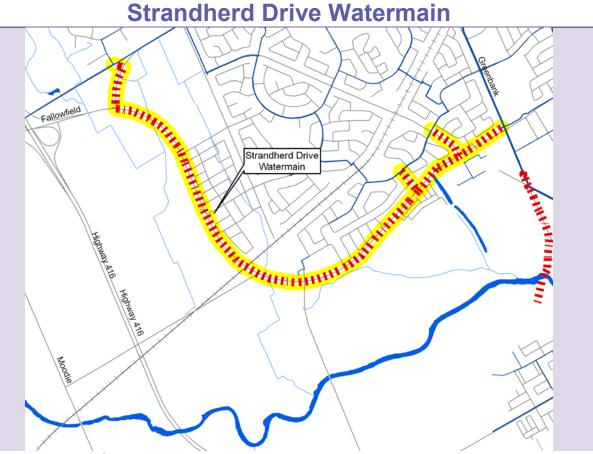
Construct 406 mm watermain along Fallowfield/Strandherd from Fallowfield/O'Keefe to Greenbank, including various connections to existing distribution system. This project is needed to support growth in the Barrhaven area north of the Jock River.
