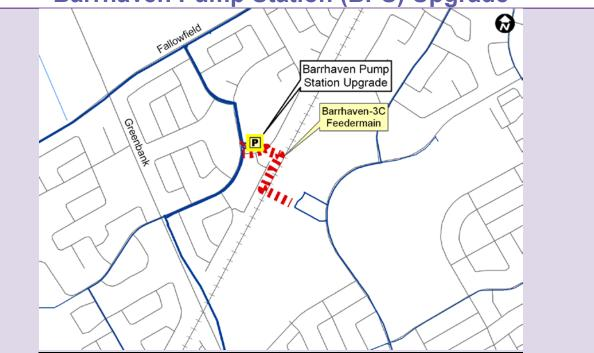
Reconfigure BPS to provide dual zone service (3C and BARR). Replace all pumping units to contribute to 2031 peak demand and back-up supply requirements for Zone 3C and Zone BARR. Upgrade back-up power.
