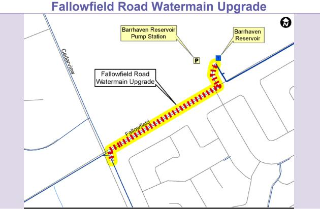
Construct 406 mm watermain along Fallowfield Rd. from Barrhaven Reservoir to Cedarview Rd. to increase effective discharge capacity available for the Barrhaven Reservoir Pump Station (BRPS). The capacity increase is needed to support growth and reliability requirements for Zone Barr.
