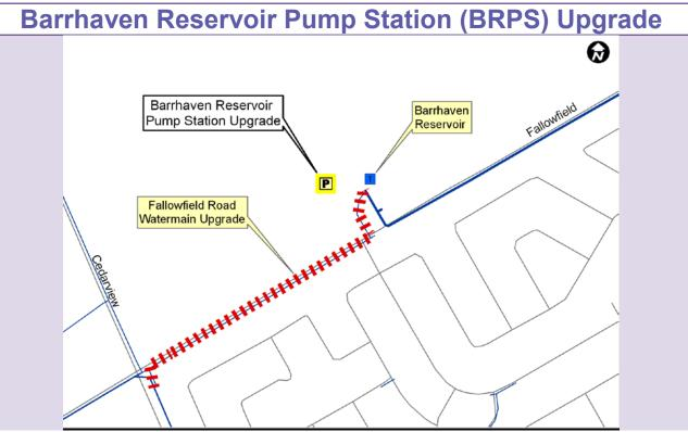
Increase pumping capacity and provide back-up powerat the BRPS (to Zone BARR) to provide adequate back-up and peaking supply demands to Zone BARR.
