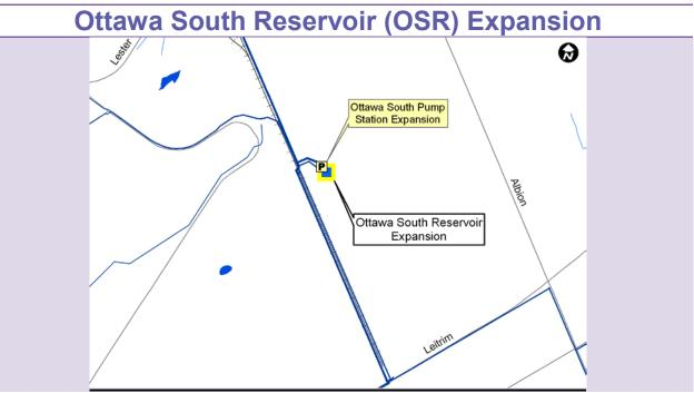
Add 16 ML of storage volume at the OSR to defer and reduce pumping expansion needs to Zone 2C from the Billings Bridge and Hurdman Bridge PSs, and defer Water Purification Plant expansion. Should land availability be an issue, a smaller increase of 12ML would be acceptable.
