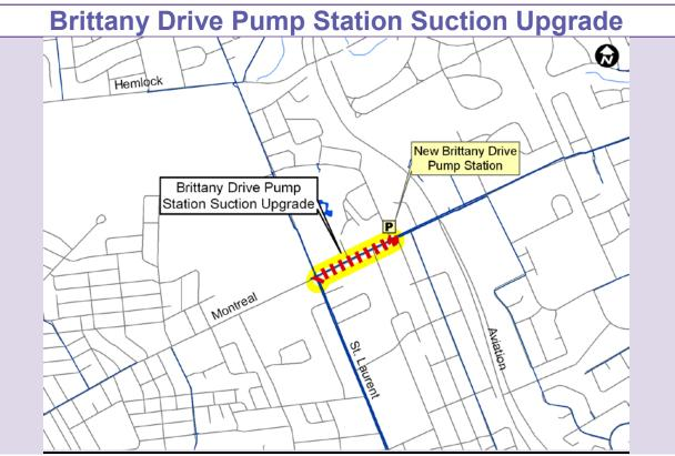
Construct 406 mm watermain along Montreal Rd. from St. Laurent Blvd. to Brittany Dr. pump station to increase suction capacity for BDPS upgrade. The upgrade is needed to support growth and improve the reliability of water supply to Zone MONT.
