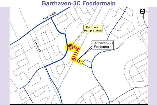
Construct 610 mm watermain from Foxfield at Holitman, across rail line and Transitway to Via Chianti Grove. The feedermain is needed to facilitate the zone reconfiguration and to meet 2031 growth and reliability requirements.
