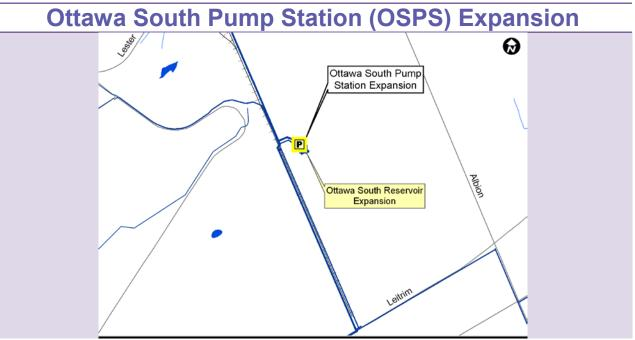
Reconfigure OSPS to provide dual zone service (3C and Uplands). Increase pumping capacity to provide 2031 peak demand to Uplands Zone and contribute to 2031 peak demand and back-up supply to Zone 3C. An expansion of the facility superstructure is required.
