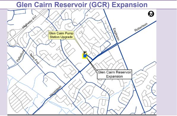
Add 17 ML storage volume at the GCR to defer and reduce pumping expansion needs to Zone 2W from the Carlington Heights PS and defer Water Purification Plant expansion.
