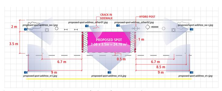
Figure 2: Required angles and naming conventions for photos of existing site conditions.
