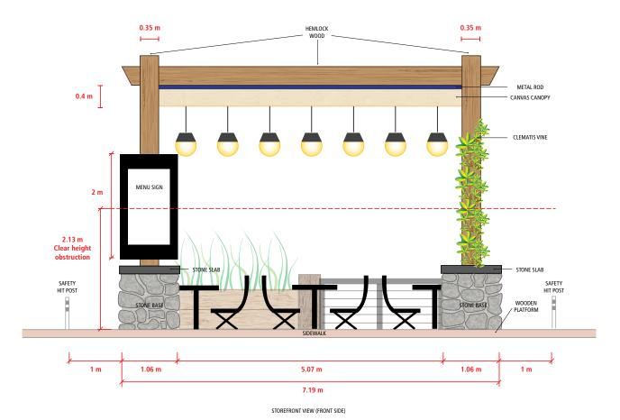
**Figure 6:** Example elevation drawing showing the storefront view of a Streetside Spot.
