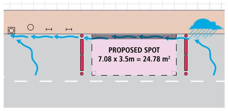
**Figure 7:** Positive drainage flow using elements in previous site plan example.
