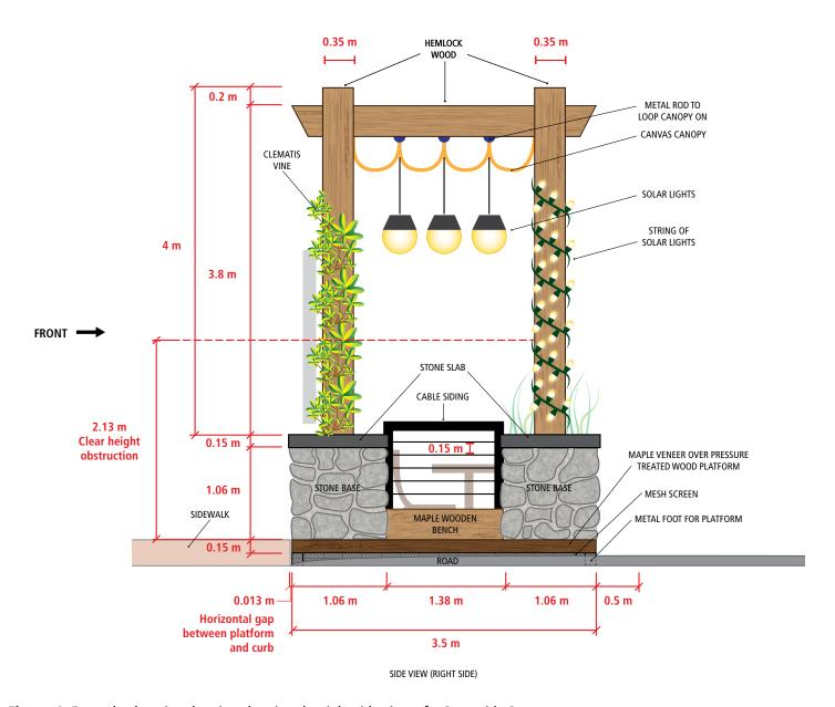
Figure 4: Example elevation drawing showing the right side view of a Streetside Spot.
