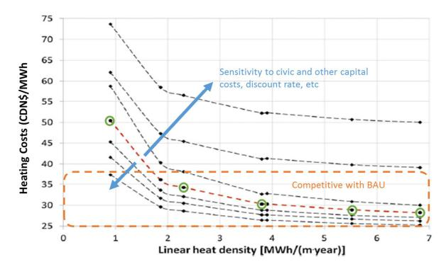
Figure 6 - High level economic viability study for a DE system in an urban environment. Adapted from Dalla Rosa<sup>5</sup>.
