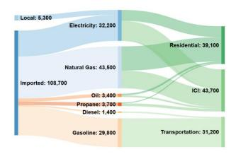
Sankey diagram showing the flow of energy by supply into usage as TJ (Source: Leidos Canada)
